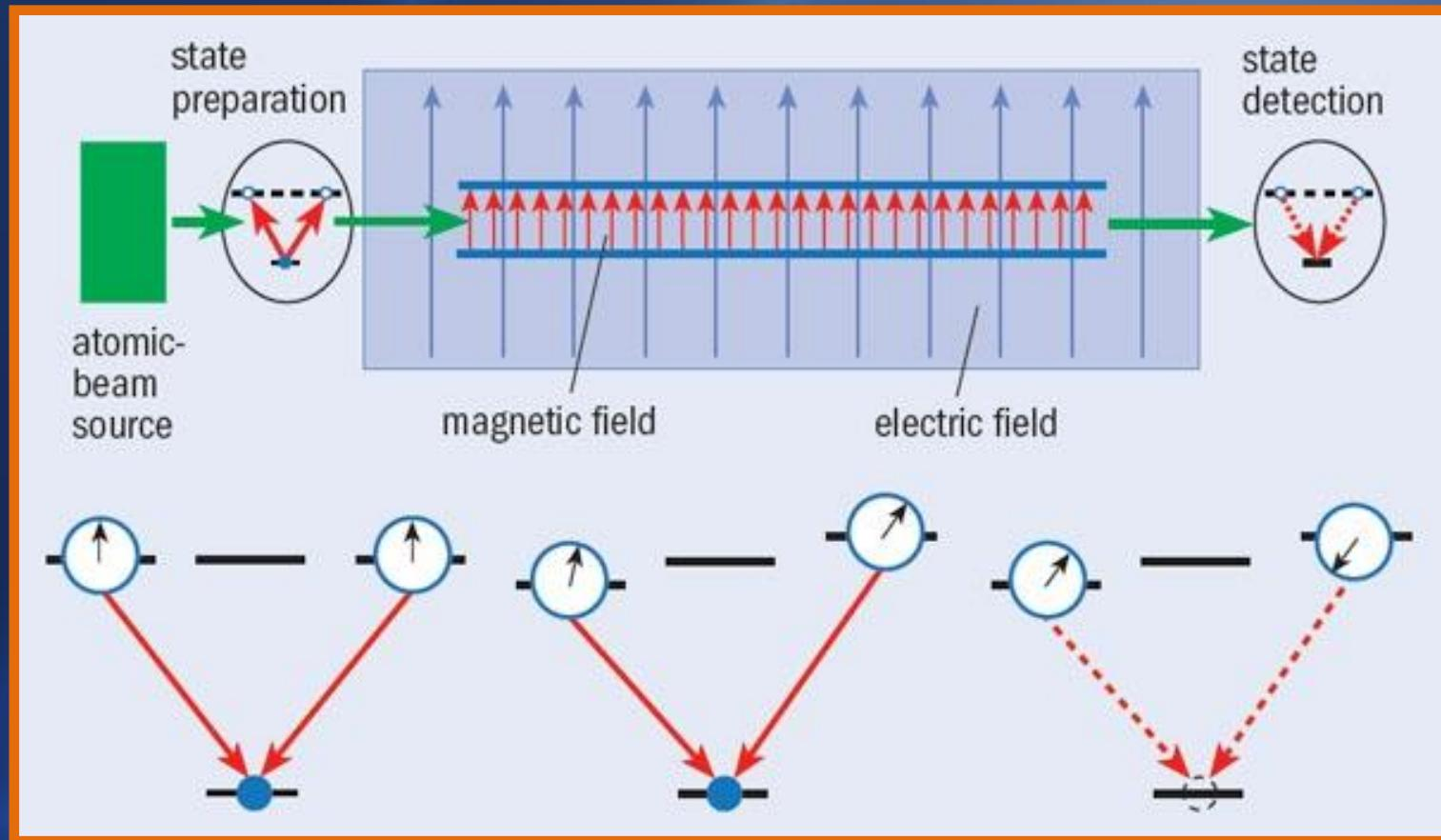
The basic structure of a beam-based electric dipole moment (EDM) experiment.
